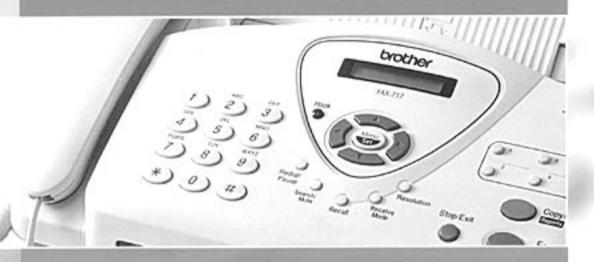
The FAX-717, with its 9,600bps modem is capable of transmitting a fax in approximately 15 seconds. And with its 512KB memory, it's also able to store up to 25 pages of incoming faxes.\*
